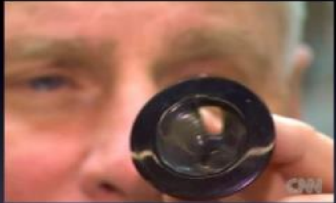
1st 3D Printed Part: eye-wash 1984 - Stereolithography
